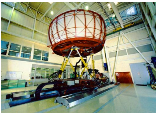
Daimler Chrysler AG: Analysis of handling and steering performance at the driving simulator in Berlin
