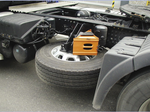
Spare wheel mount on truck frame
