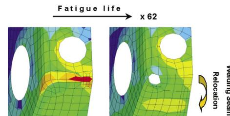
*Improved fatigue life as result of relocated weld*
