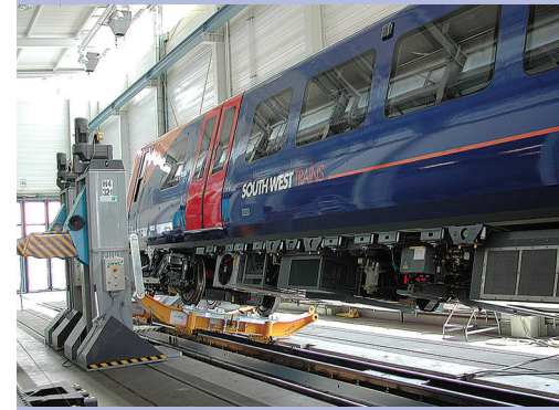
Sway Test in the Validation Center Wildenrath
