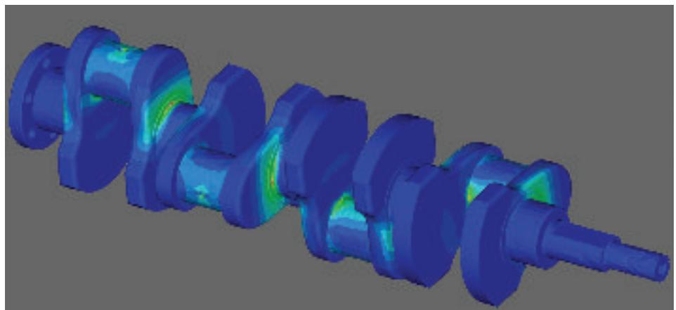
*Fig. 1: Mises's stresses of a crankshaft at a high revolution speed calculated with NASTRAN. SIMPACK's LOADS interface combination with NASTRAN and FEMAT exactly produces the same result.*
