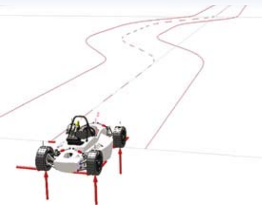
Fig. 4: Multi-body simulation of the busstop
