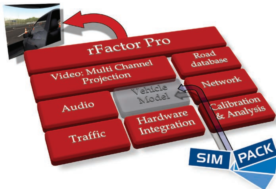
Fig. 1: The SIMPACK interface for rFactor Pro
