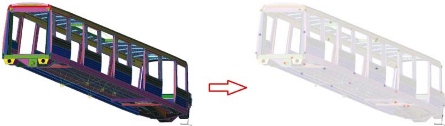
Fig. 2: Master DOFs selection for dynamic reduction of carbody (FE Mesh -> nodes of super element)
