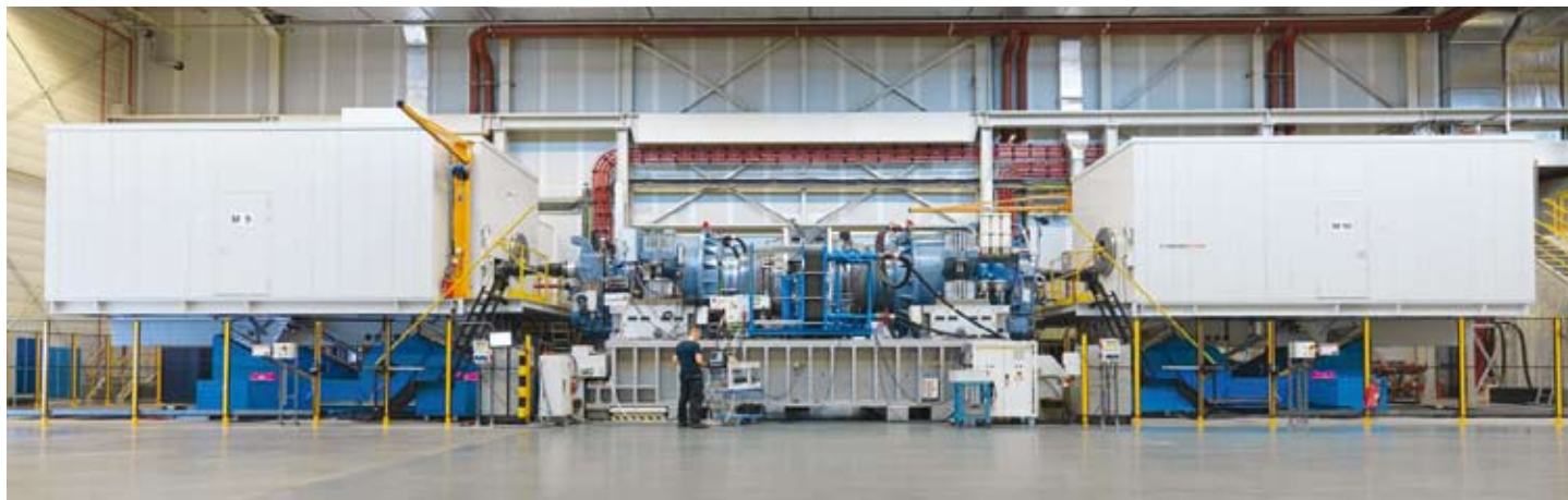
Fig. 1: 13.2 MW dynamic test rig with REpower's 6 MW gearbox in a back-to-back configuration
