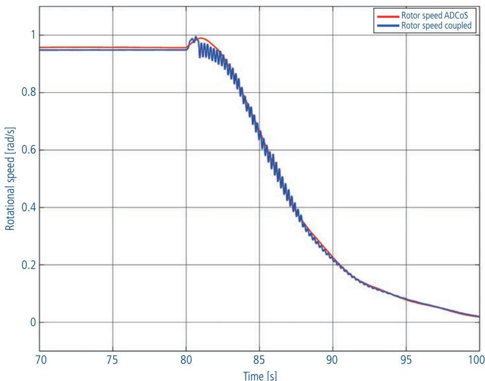
Fig 5: Comparison of rotor speed of a coupled and a pure ADCoS simulation of an emergency shutdown with loss of electrical network connection
