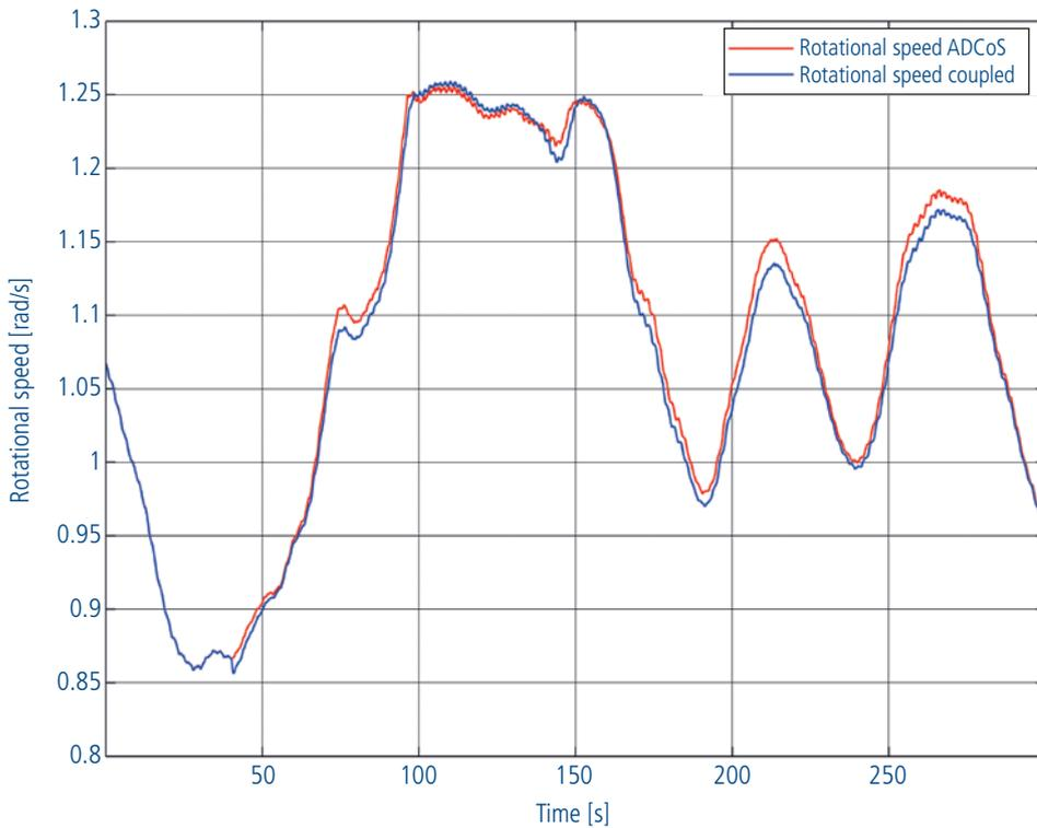
Fig 2: Comparison of rotor speed in both a coupled and a pure ADCoS simulation
