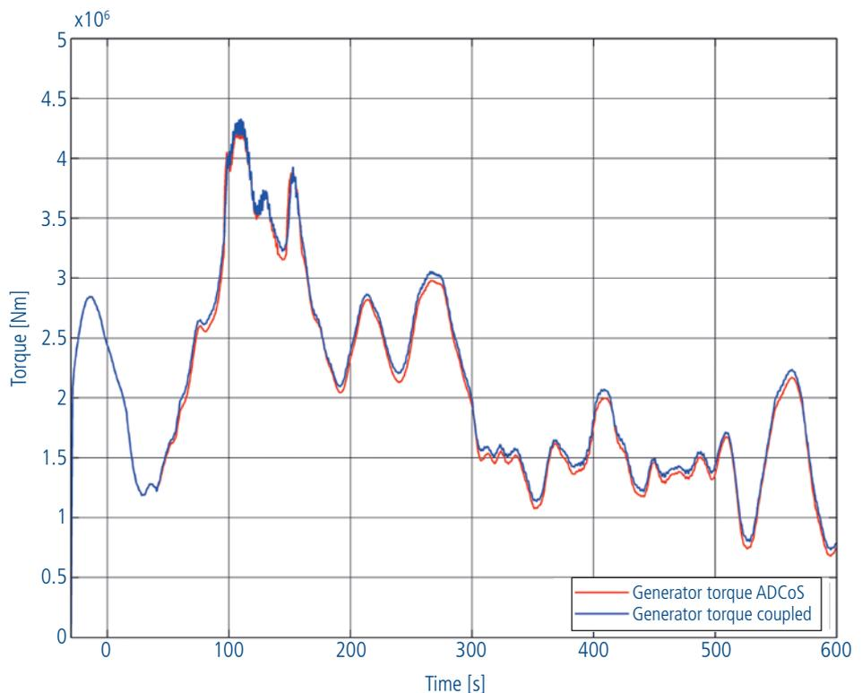
Fig 3: Comparison of generator torque of a coupled and a pure ADCoS simulation
