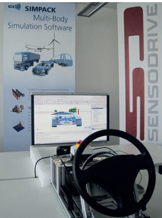
Fig. 2: SIMPACK Realtime desktop driving simulator using a high precision SENSODRIVE steering wheel
