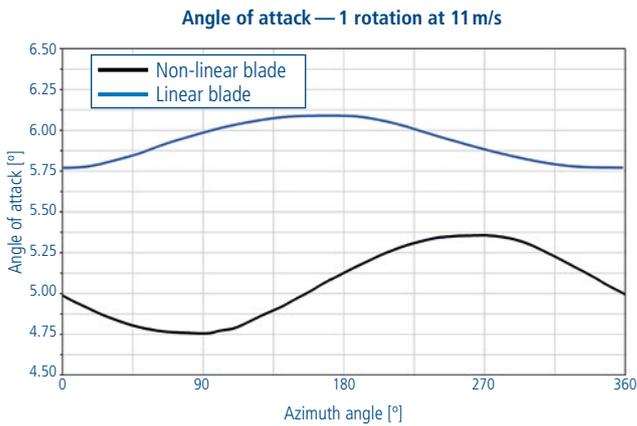
Fig. 9: Angle of attack over azimuth angle, 0° = pointing upwards
