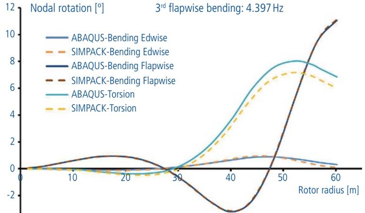
Fig 5: Normalized nodal rotation for the 3<sup>rd</sup> flapwise bending mode
