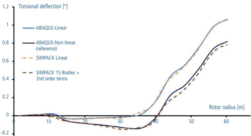
Fig 4: Torsional deflection due to distributed lift forces near rated power
