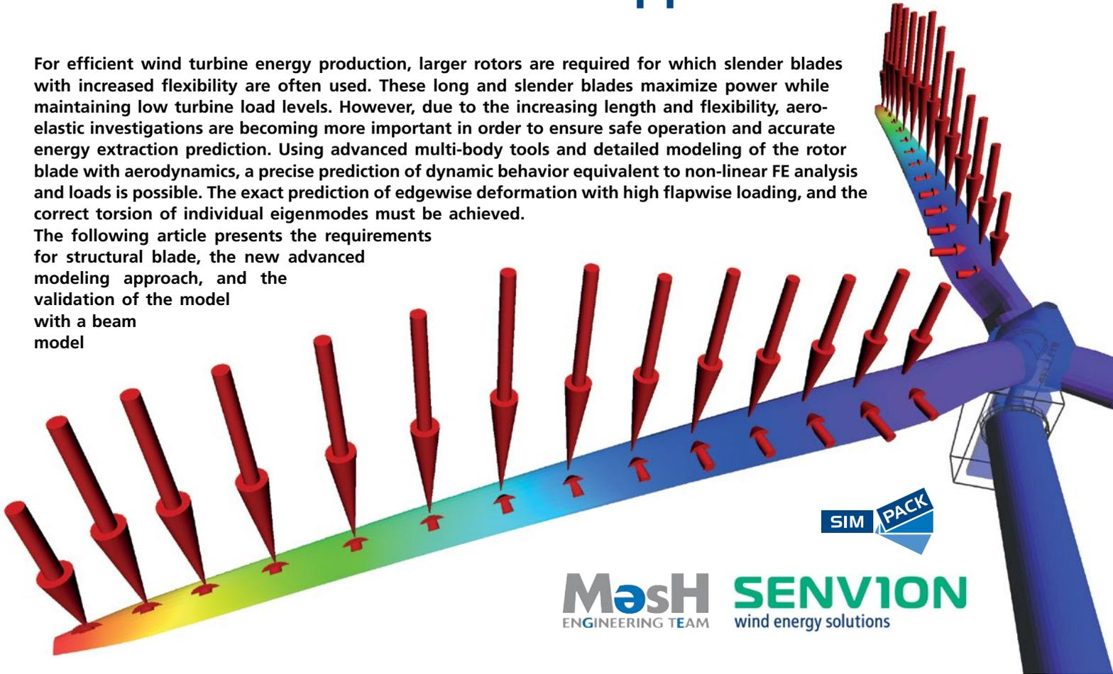
set in the FE code ABAQUS. Data from the UpWind 61.5m blade was used. Additionally, impact on aeroelastic performances simulations with the complete rotor were carried out, and a comparison between traditional modeling approaches and the new advanced method is offered.
