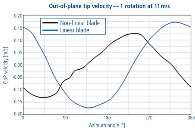
Fig. 8: Out-of-plane tip velocity over azimuth angle, 0° = pointing upwards
