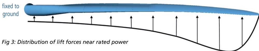
Fig 3: Distribution of lift forces near rated power
