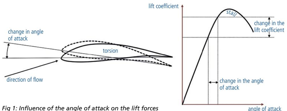
Fig 1: Influence of the angle of attack on the lift forces
