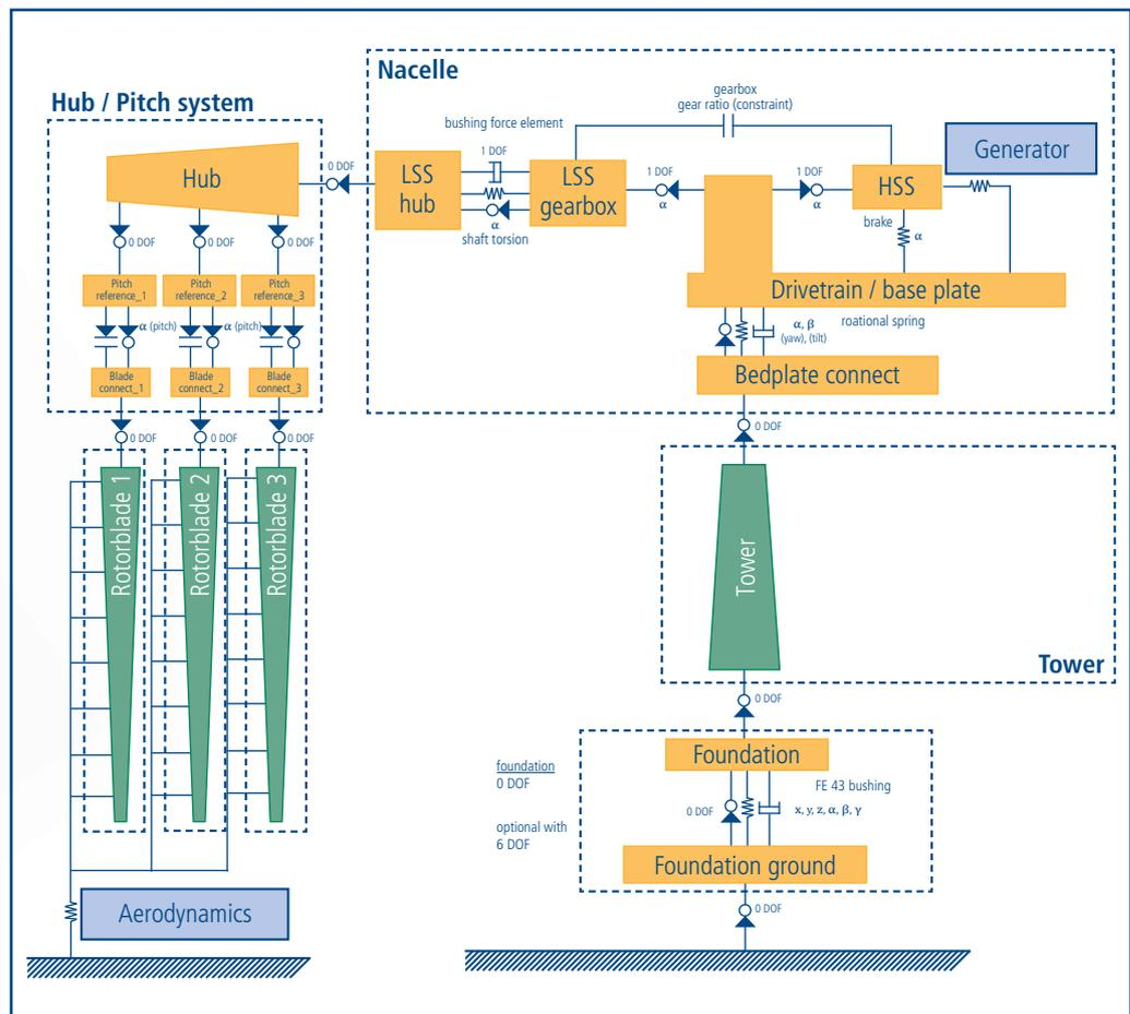
Fig. 6: Wind turbine model considering the linear and non-linear rotor blade model
