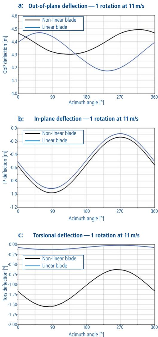
Fig. 7: Tip deflection over azimuth angle, 0° = pointing upwards: out-of-plane deflection (a), in-plane deflection (b), and torsional deflection (c)
