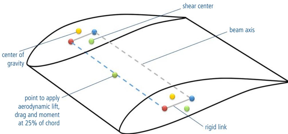
Fig 2: Advanced 3D beam structure
