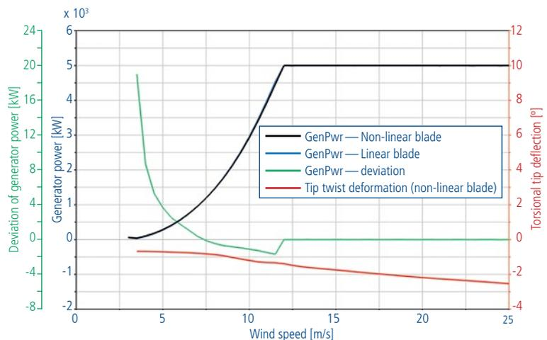
Fig. 10: Power curve and torsional tip deflection of the UpWind turbine
