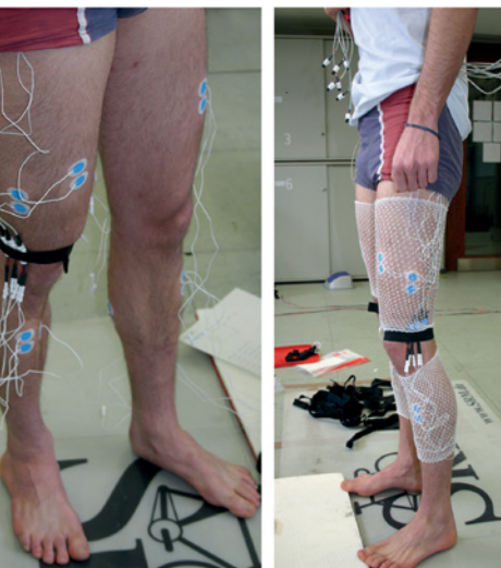
Fig. 7: Muscle activation patterns were measured through electromyography (EMG)
