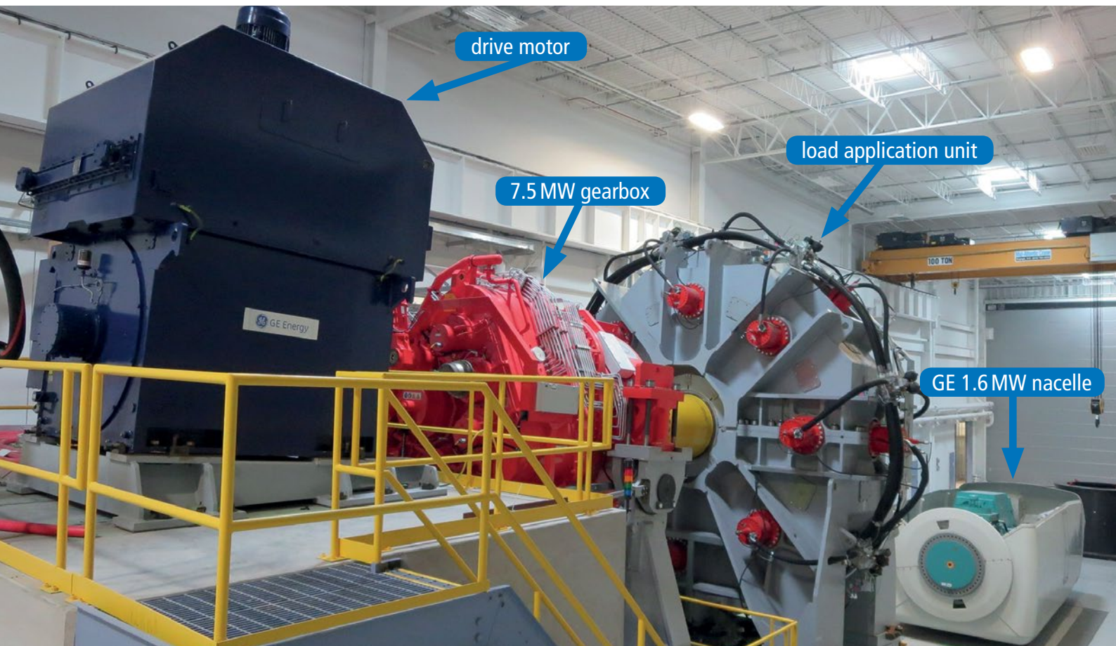
Fig. 1: Clemson University's 7.5 MW test bay showing the drive motor, gearbox, load application unit, and nacelle
