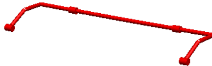
Stabilisor Bar: Free/Free Mode Shape + Freq. Resp. Modes + Bushings
