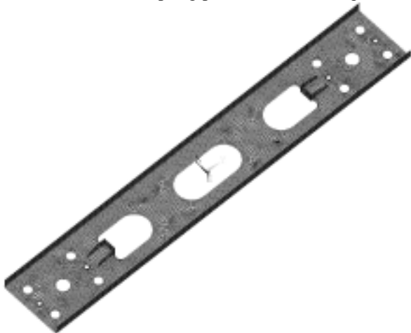
Figure 3. The FE-model of spring plank
